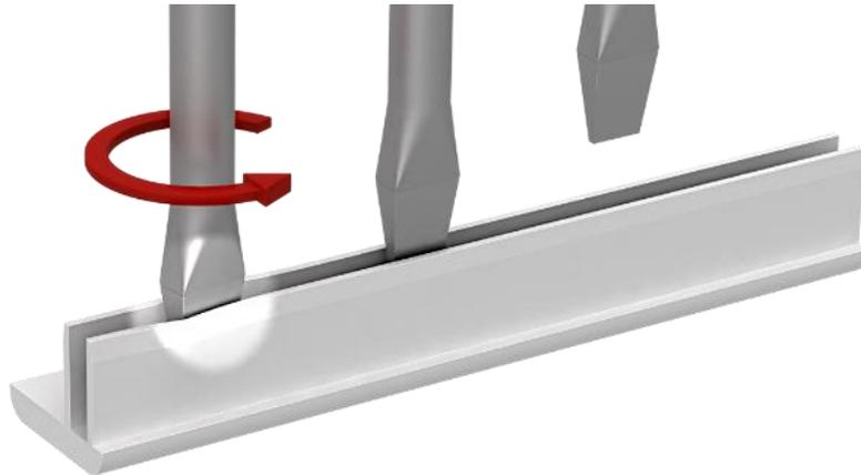
Insert the front pane and the connectors. Spread the connectors slightly with a screwdriver before inserting so that they are stuck firmly in the housing frame. Check that the connectors are fixed so tightly after insertion that they cannot be removed without tools (lever tools).
