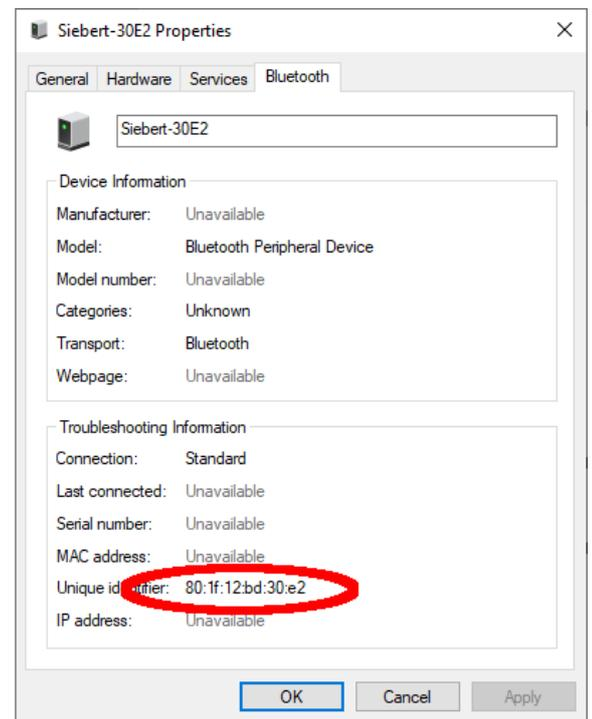
Open the tab 'Services' of the properties dialogue box. The Bluetooth feature 'serial connection (SPP)' has to be activated for the display. The virtual COM port that is used for communication is specified thereafter.
